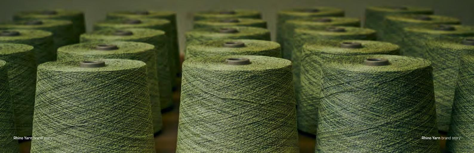
We've never been afraid to try new things. So, in 2001 our yarn technologists began developing composite yarn structures with a stainless steel core. As soon as we knew we were able to process and spin steel to incredibly fine grades whilst achieving high-cut performance, we knew we were on to something.
